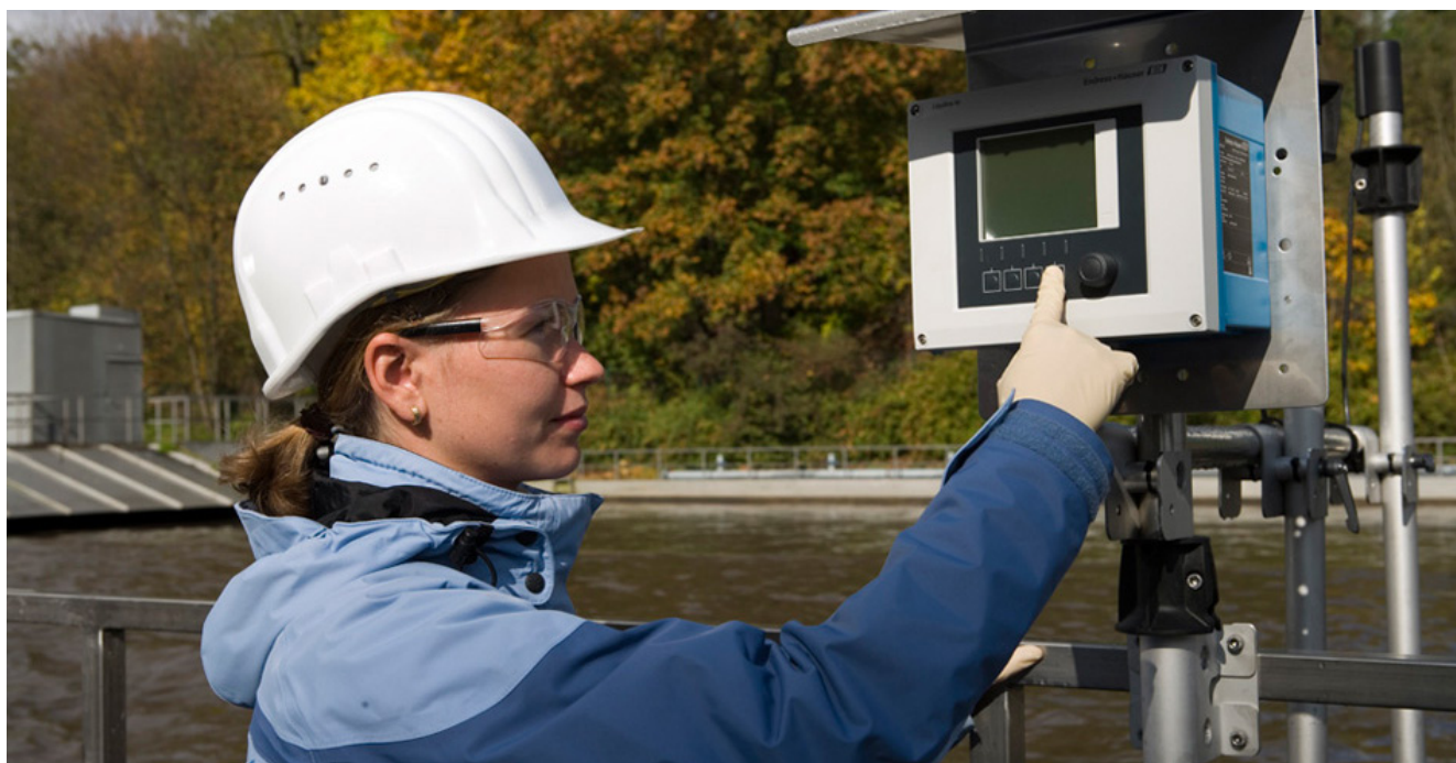
Online analytics with the Liquiline CM44x transmitter is the basis for further optimization in biological treatment
